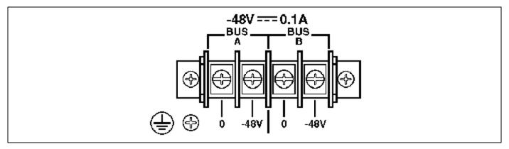
Figure 4.1: Terminal Block Assembly and Grounding Screw (DC Units Only)
